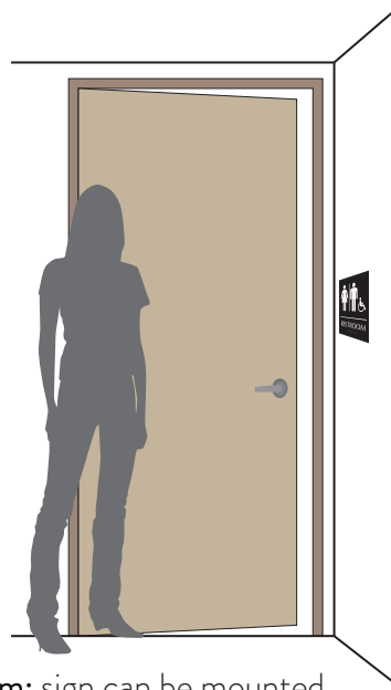
No room: sign can be mounted on nearest adjacent wall.
